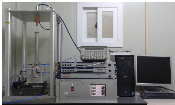
Figure 4: A picture of the wire test stand. A BPM translation stage with wire holder, a motor controller, BPM electronics, and a control computer are shown.
