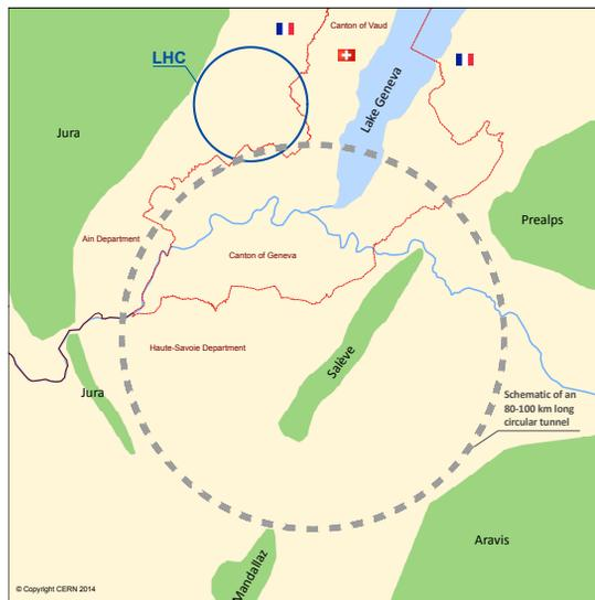
Figure 4: Schematic view of the FCC ring in the Geneva area (copyright CERN 2014).
