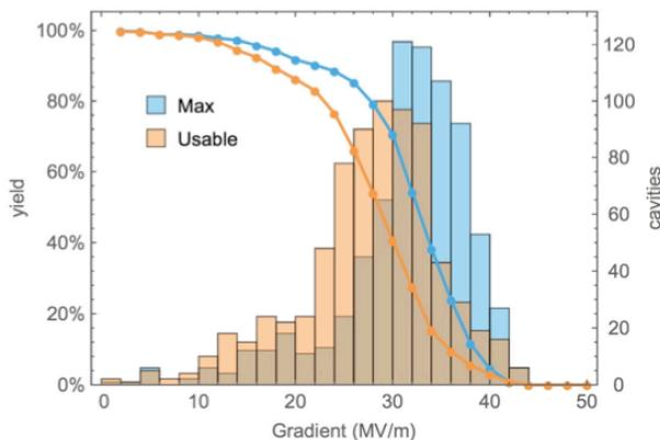
Figure 7: Maximum and usable gradients of superconducting XFEL cavities. Many of the cavities fulfill the ILC requirements (courtesy European XFEL).
