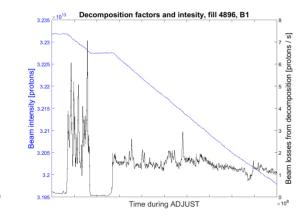
Figure 5: Beam intensity (blue) and losses from decomposition (black).
