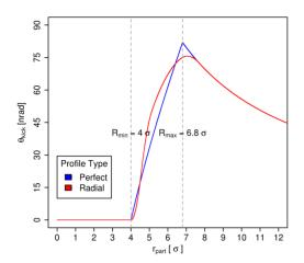
Figure 4: Kick strength for perfect and radial electron density profiles.
