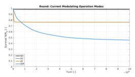
Figure 5: Halo survival fraction as a function of turn for different beam modes in HL-LHC at the round beam position.
