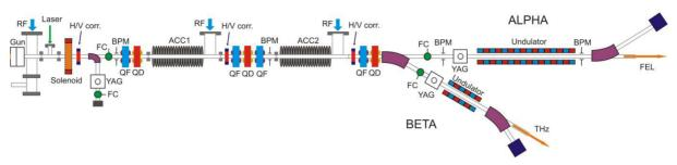
Figure 1: The schematic layout of AREAL linear accelerator.
