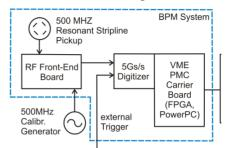
Figure 3: The BPM system block scheme.
