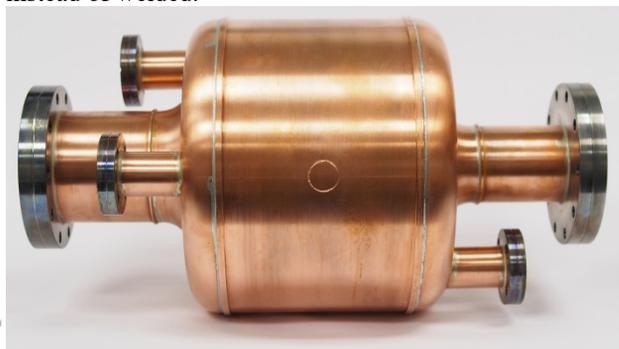
Figure 4: The copper prototype cavity
