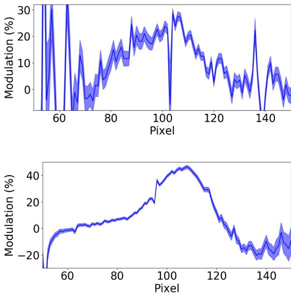
Figure 4: Unprocessed EO signal in the presence of an electron bunch, including pixel defects (e.g. pixel 104 in upper plot), using EOS v1 (top), and EOS v2 (bottom). The blue lines mark the change of the detected laser intensity due to the presence of an electron bunch. The error bands are due to the electronic noise. The increased modulation for EOS v2 is due to improvements in the alignment and the new design.
