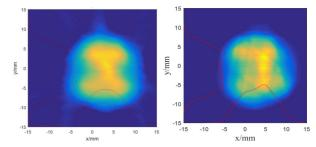
Figure 7: Reconstructed 2D beam profile. Left: ART algorithm with 33 projections, right: MENT algorithm with 5 projections.
