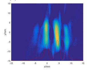
Figure 8: Reconstructed profile with ART algorithm from 33 projection with the mask inserted.
