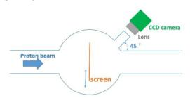
Figure 1: Schematic diagram of profile monitor based on scintillator screen.
