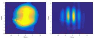
Figure 5: Beam profile monitored by scintillator screen. left: w/o mask, right: with mask inserted.
