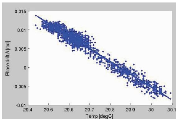
Figure 1: BPM measured phase affected by environment temperatures.
