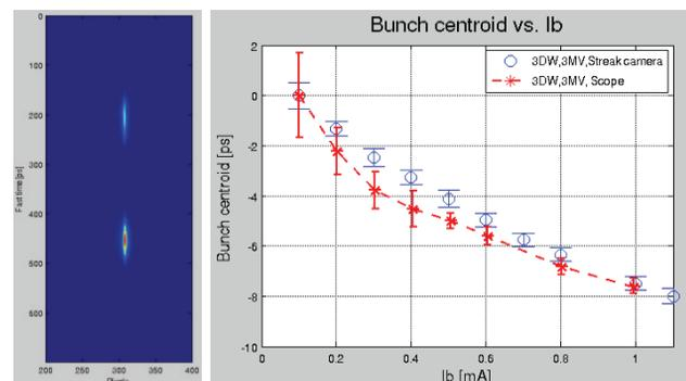
Figure 2: (left) Streak camera synchronous phase measurement with reference bunches; (right) Measured single bunch phase drifts with bunch current.
