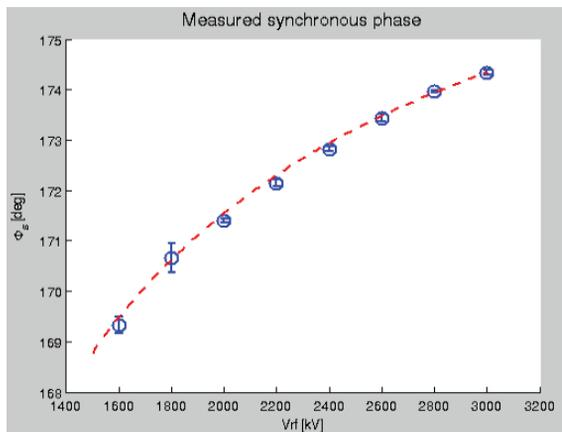
Figure 3: Measured synchronous phase drift with RF voltage in bare lattice. Red dash lines is the calculated synchronous phase based on fitted  $U_{sr}$  of 297 kV.
