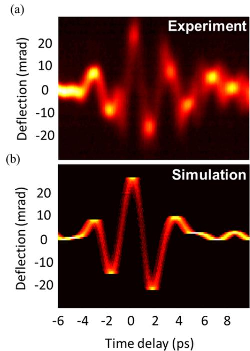
Figure 2: (a) Transverse deflection as a function of delay between THz-field and electron bunch; (b) Simulated deflection trace [5].
