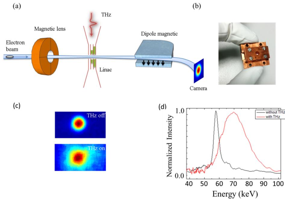
Figure 1: (a) Acceleration of an electron bunch from a 57 keV DC-gun using a multiple layer THz acceleration device with dipole magnet for energy measurement on MCP; (b) THz acceleration device; (c) Electron beam with and without THz acceleration on the detector; (d) Electron energy spectrum without (black) and with THz pulse (red).
