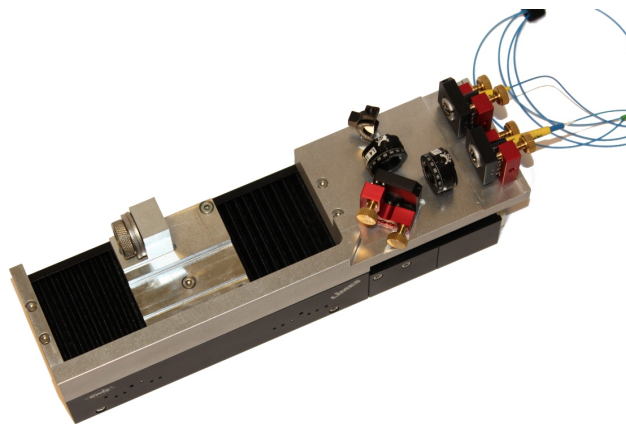
Figure 4: The delay stage is mounted on the linear stepper motor. For calibration purpose an encoder can be attached to the stepper motor as well (not shown in the photo).
