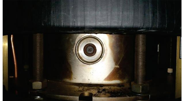
Figure 4: Failed second cavity connection attributed to failed 50-ohm load.
