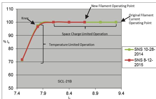
Figure 6: Typical emission graph. The Y-Axis is cathode emission percentage. The X-axis is filament current in amperes.
