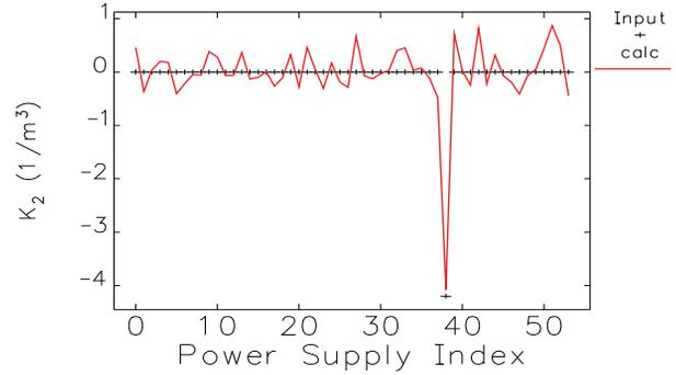
Figure 6: The cross shows the index number (39) of the altered circuit with  $\Delta K_2 = 4.2m^{-3}$ , and the red curve is the error identified by the algorithm.
