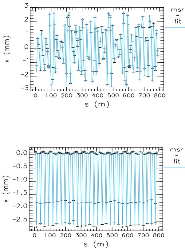
Figure 1: The measured and the fitted orbit. Top: The fitted bending angle is 0.18 mr. Bottom: The fitted momentum offset is -0.6%.
