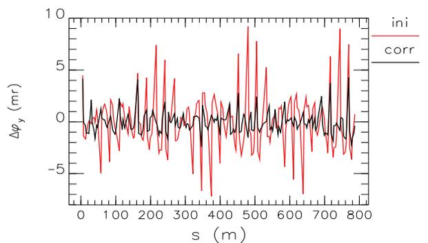
Figure 3: The initial and the residual phase error after one round of correction. One plane is shown only.
