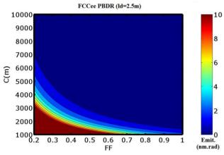
Figure 3: Scaling of emittance with filling factor and circumference.
