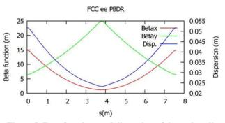
Figure 5: Beta functions and dispersion of the main cell.
