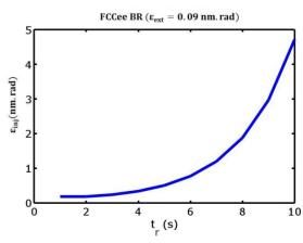
Figure 2: Injection emittance of booster ring with ramping time.
