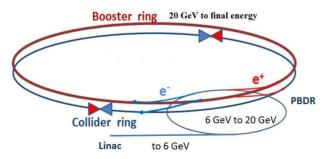
Figure 1: Layout of FCC ee injector complex.
