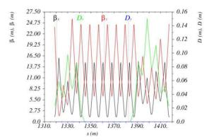
Figure 6: Straight section optics of PBDR.
