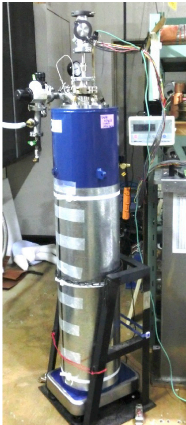
Figure 10: Galvanized iron sheets are wrapped around the cryostat to reduce the stray magnetic field.
