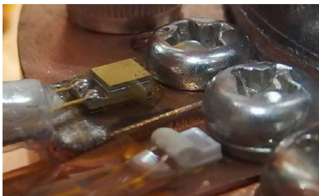
Figure 4: Mounted temperature sensors. Left: CERNOX Model: CX-1030-SD-1.4L. Right: pt100
