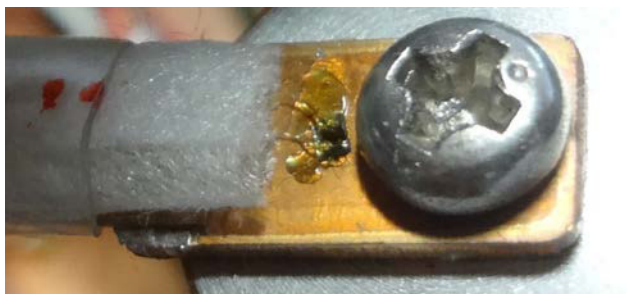
Figure 5: Mounted CERNOX sensor CX-1030-BG-HT.
