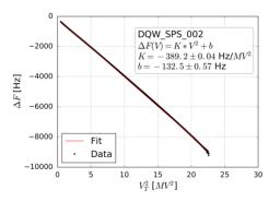
Figure 6: Lorentz Force Detuning data fitting for cavity 002.
