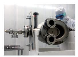
Figure 1: One of the two DQW\_SPS crab cavities during clean room assembly (ISO4).
