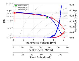
Figure 4: First performance results (at 1.9 K) for the DQW crab cavities to be installed the SPS test.
