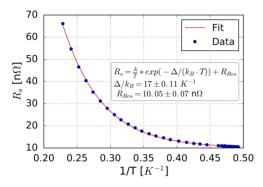
Figure 5: Surface resistance data fitting for cavity 001.
