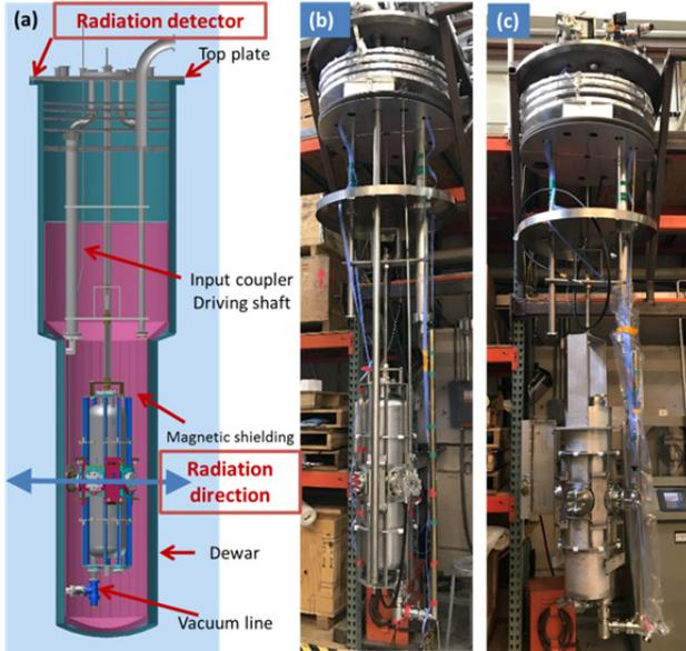
Figure 3: The HWR-1 cavity on the insert. (a) Diagram of the HWR on the RF insert for the vertical tests with the view of the Dewar and magnetic-field shielding. (b) Photograph of the HWR-1 bare-cavity on the insert. (c) Photograph of the HWR-1 dressed-cavity on the insert.
