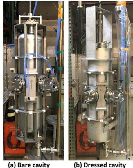
Figure 2: Photograph of (a) the bare HWR-1 cavity (b) the dressed HWR-1 cavity. Both cavities are installed with the handling frames.
