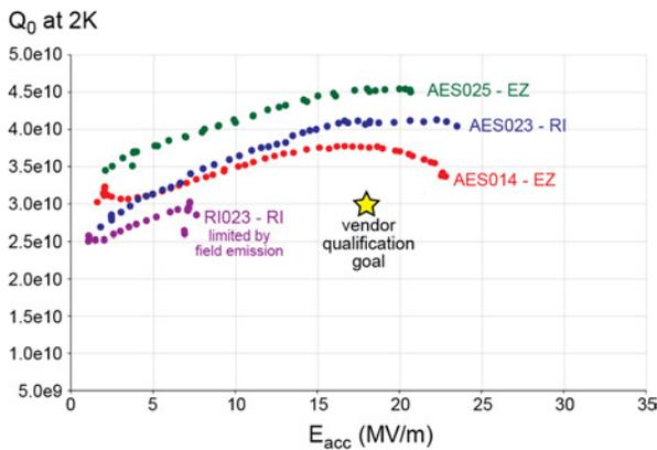
Figure 1: Vertical test results of four TESLA cavities after N-doping at RI and EZ, respectively. The cavity ID and vendor are denoted next to the data.  $Q_0$ -values are corrected for the cavity flange losses (stainless steel), which will not be present in a cryomodule.
