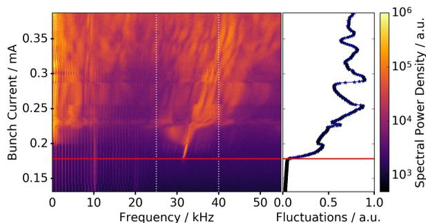
Figure 1: Temporal emission spectrum of THz intensity as function of decreasing bunch current. The red line indicates start of the fluctuations due to the micro-bunching instability. In the right panel the sum of the fluctuation power in frequency range 25–40 kHz shows a strong increase at the threshold current.
