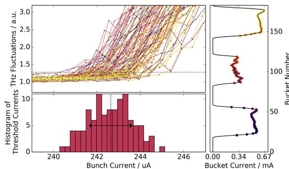
Figure 3: THz fluctuations as function of bunch current for all bunches in a multi-bunch fill. The vertical (dotted) line in the histogram of the threshold currents of each bunch (lower panel) indicates the average of the threshold currents  $\mu(I_{th})$  while the horizontal arrows indicate the spread (standard deviation) of threshold currents  $\sigma(I_{th})$ . The filling pattern at the start of the decay is indicated in the right plot.
