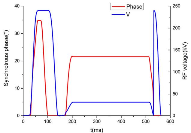
Figure 12: Voltage program during the whole process.
