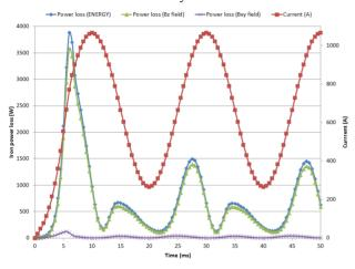
Figure 2: Eddy current losses in the yoke.
