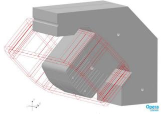
Figure 1: Geometry of 1/8<sup>th</sup> of the yoke.
