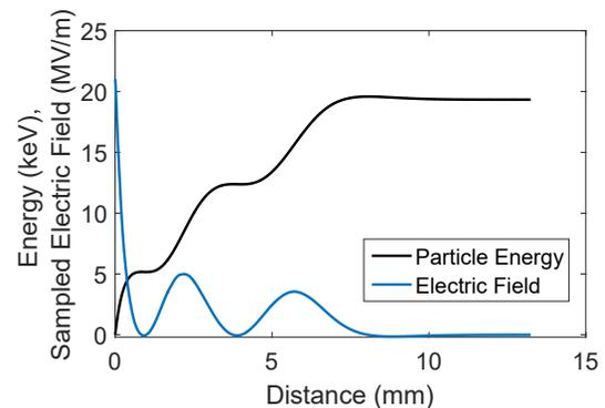
Figure 3: Single particle simulation of for optimal energy gain, with both the particle energy and the sampled electric field show vs. distance. The RF gun requires 1.5 kW of RF power to achieve this field strength.
