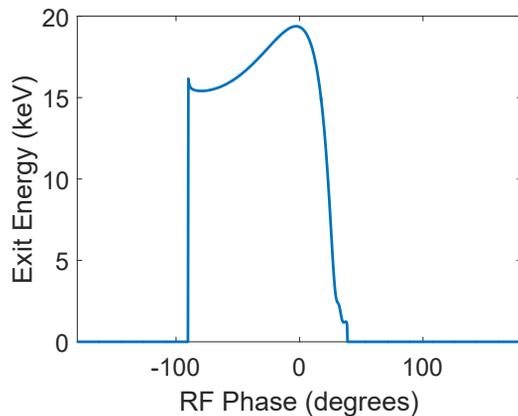
Figure 4: The exit energy as a function of the launch phase for the RF gun. The phase is reference with respect to the peak energy gain for the single particle shown in Fig. 3.
