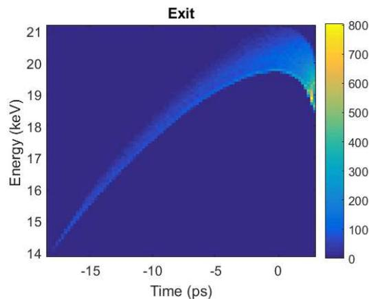
Figure 5: The longitudinal phase space of the electron bunch at gun exit in time vs electron energy.
