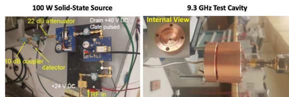
Figure 6: (left) Assembly of the three stage 100 W amplifier chain. Isolators are placed between stages. (right) 9.3 GHz cavity powered by solid-state source. The cavity is critically coupled from one side and weakly coupled from the other side using coaxial probes, loaded Q factor is 3200.
