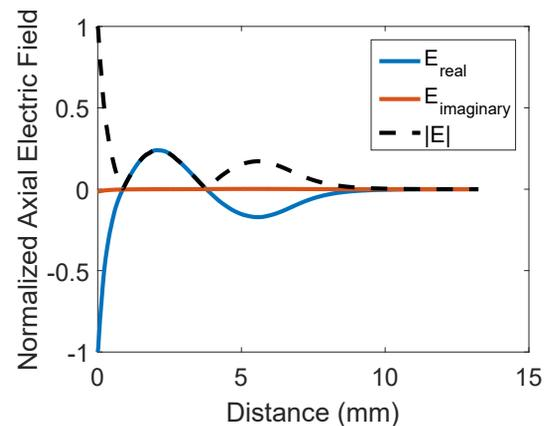
Figure 2: On-axis electric field for RF electron gun. The field is strongly peaked on the cathode and drops rapidly as the cell length increases.
