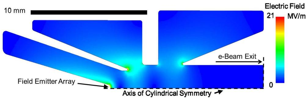
Figure 1: Electric field distribution in the RF gun.
