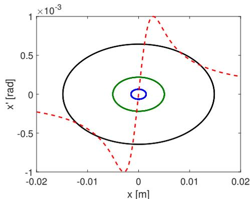
Figure 1: Initial distribution of spectator particles in horizontal phase space. Each ellipse contains 1000 equidistantly distributed particles. The dashed line is an overlay of the beam's self-field.
