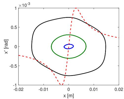
Figure 2: Matched beam after ten turns. Initial ellipses exhibit different angles, depending on whether particles see a positive or a negative self-field gradient and the respective incoherent tune-shifts.
