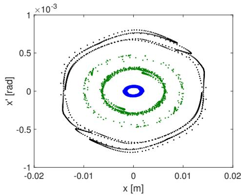
Figure 4: Hor. phase space after 1000 turns with  $B_{mag} = 1.083$ . Particles close to field maximum experience strong filamentation and split into two ellipses.
