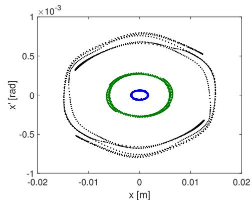
Figure 3: Phase space ellipses for a matched beam after 1000 turns. Smearing of ellipses is observed.
