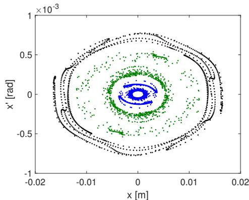
Figure 5: Hor. phase space after 1000 turns with  $B_{mag} = 1.25$ . Particles close to beam core form eye-shaped structures.
