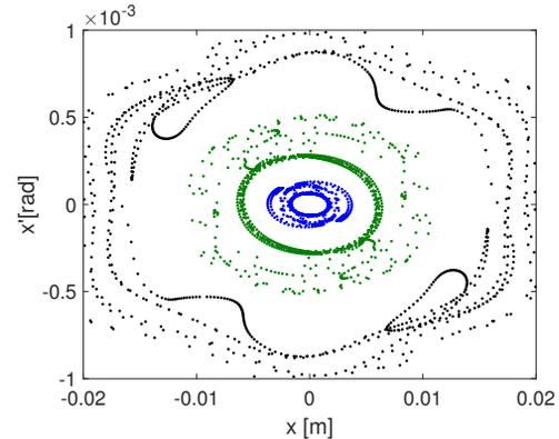
Figure 6: Beam mismatch with  $B_{mag} = 1.083$  after 1000 turns. Planes are coupled by a quadrupole with a  $1^\circ$  skew angle.
