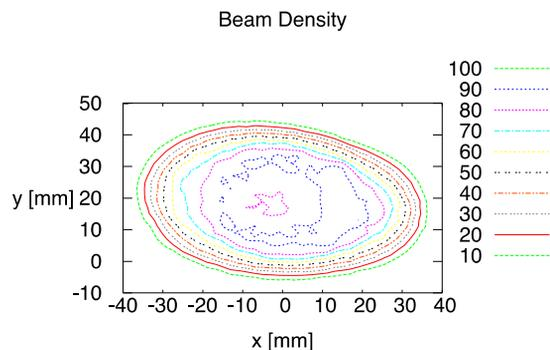
Figure 2: Footprint of simulated self-consistent beam at target. The density is very uniform, as it should be for a self-consistent beam.
