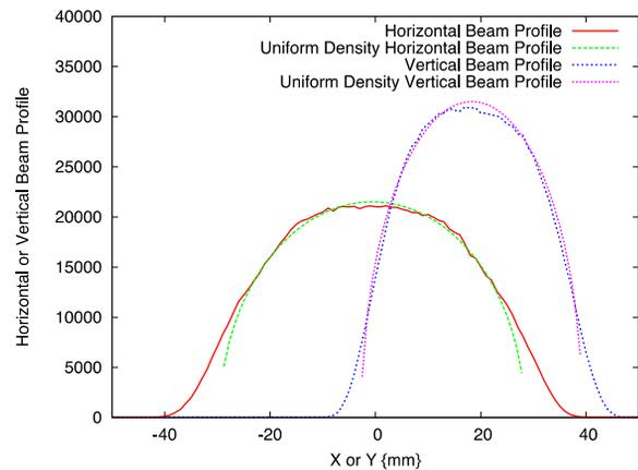
Figure 1: Comparison of horizontal and vertical accumulated beam profiles from simulation with those for an exactly self-consistent beam. Agreement is excellent except at the edges, where the effect of the finite size of linac beam at the foil causes some spreading.
