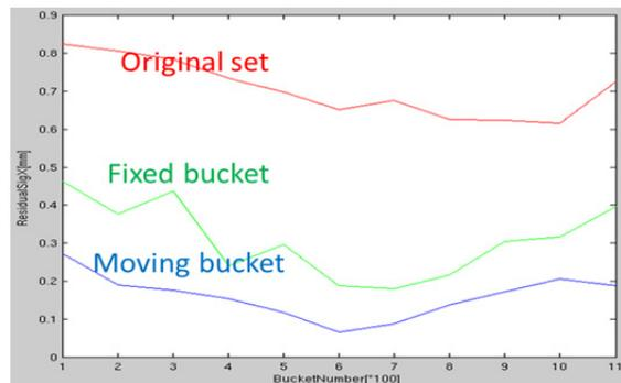
Figure 5: BPM TBT data RMS value dependence on injection bucket after local and global optimization.
