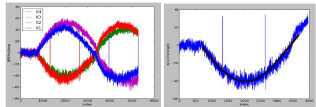
Figure 3: Bunch by bunch position measurement in four turns (left) and kicker waveform fitting (right).
