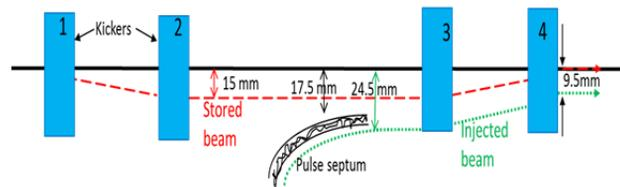
Figure 1: Cartoon of beam position during injection at SR injection straight section.
