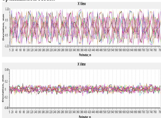
Figure 4: Top off injection transition from BPM TBT data before (top) and after (bottom) kicker optimization.
