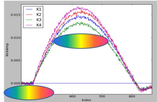
Figure 2: Bunch train distribution relative to kicker waveform during kicker excitation.
