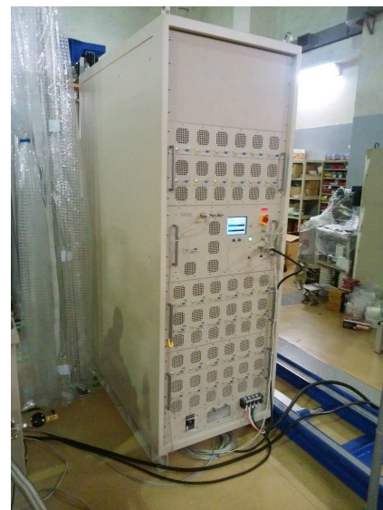
Figure 2: Solid-state amplifier developed for R&D program in Yamagata University.
