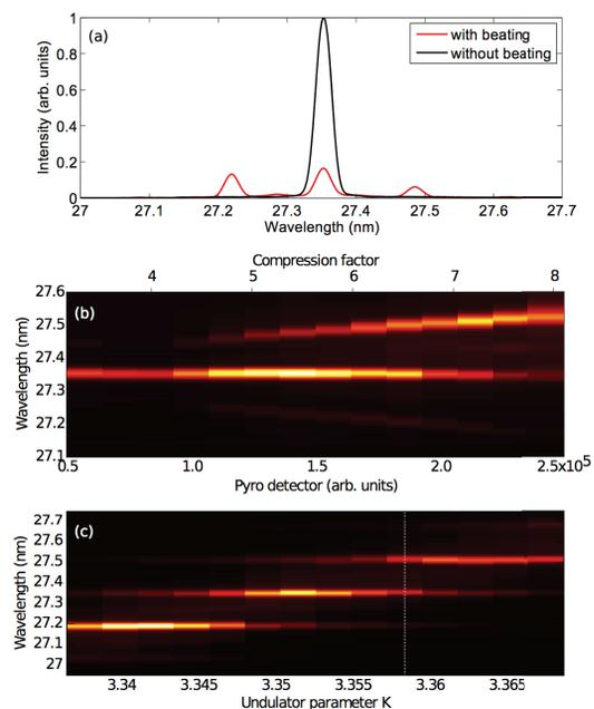
Figure 3: (a) FEL spectra in the nominal LH configuration (black line) and in the LH beating configuration (red line) (average over 20 shots). (b) Evolution of the FEL sideband position versus compression factor. The pyro detector signal is proportional to the compression factor. (c) FEL emission spectra versus radiator tuning.
