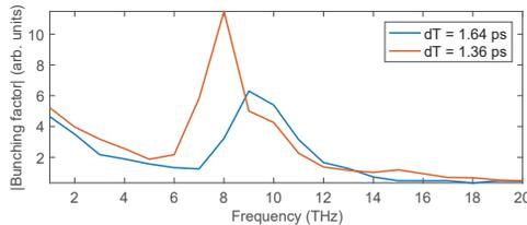
Figure 4: Fourier transform of the current profile of the electron beam at the end of the linac for two delays of the LH beating.
