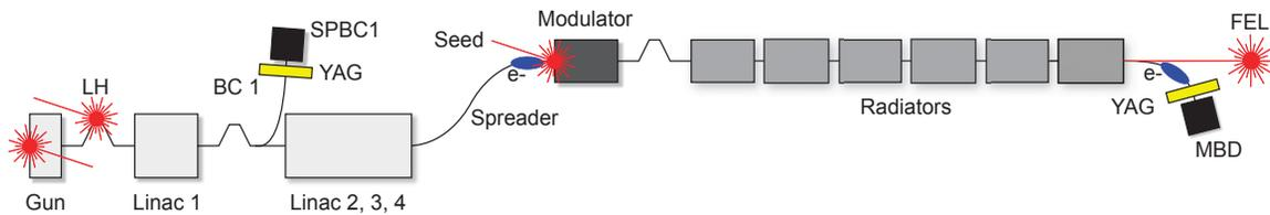
Figure 1: FERMI FEL-1 layout. After being extracted from the photoinjector (GUN), the electron bunches pass through the laser heater (LH) section and are then compressed in the bunch compressor (BC1). Following an acceleration to 1.0 – 1.5 GeV, the electron bunches are sent to the FEL-1 undulators.
