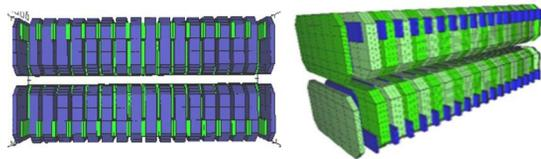
Figure 2: Prototype design of the undulator U18 (left) and U15 (right) with 7 periods, using RADIA code with IGOR Pro as front end.
