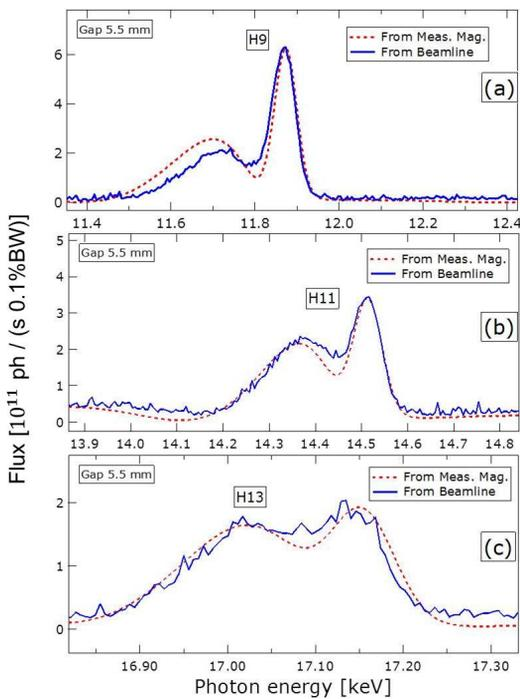
Figure 4: Normalized spectra measured on the beamline (non absolute) and calculated from magnetic measurements at 5.5 mm gap through a 0.05 mm x 0.05 mm aperture at a distance of 20.3 m from the undulator. Electron beam parameters same as of Fig. 3 caption, but with  $\beta_x = 8.906 m$ ,  $\beta_z = 7.216 m$ ,  $\alpha_x = -1.296 rad$ ,  $\alpha_z = -1.477 rad$ . (a): 9<sup>th</sup> harmonic, (b): 11<sup>th</sup>, and (c): 13<sup>th</sup> harmonic.
