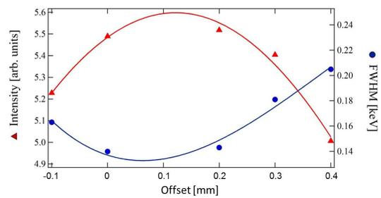
Figure 5: Intensity and Full Width Half Maximum (FWHM) of the 11<sup>th</sup> harmonic as a function of the offset that varied from -0.1 mm up to 0.4 mm.
