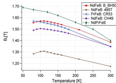
Figure 1: Magnet grades remanent field versus temperature [6, 7].
