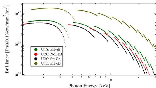
Figure 3: Brilliance in logarithmic scale, with beam energy 2.75 GeV, energy spread rms 0.01 %, beam current of 0.5 A, horizontal emittance of 3.9 nm, vertical emittance of 0.039 nm,  $\beta_x = 5.577$  m,  $\beta_z = 8.034$  m,  $\alpha_x = -1.296$  rad,  $\alpha_z = -1.477$  rad.
