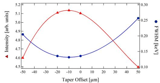
Figure 6: Intensity and Full Width Half Maximum (FWHM) of the 11<sup>th</sup> harmonic as a function of the taper offset.
