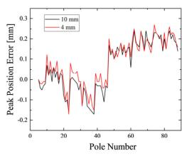
Figure 6: Peak position error in the PCU2.
