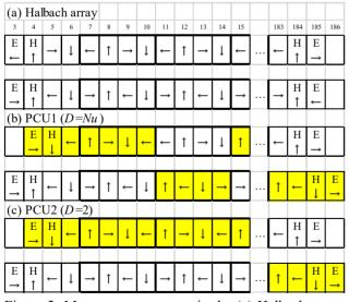
Figure 2: Magnet arrangements in the (a) Halbach array, (b) PCU1, and (c) PCU2. Here white box and the arrow inside indicate the magnet and its magnetization direction. The yellow magnets in PCU indicate magnets has been moved from the original Halbach array. Symbol H and Eindicate the special end magnets having the thickness of 4 and 4.8 mm, respectively.
