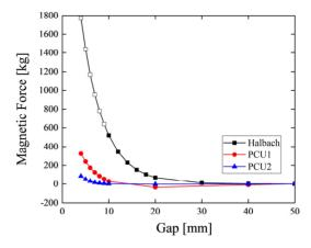
Figure 3: Magnetic force measured by the strain-gauge load cell in Halbach (black square measured, white square extrapolated), PCU1 (red circle) and PCU2 (blue triangle).
