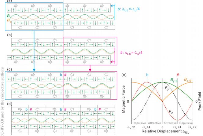
Figure 1: Conceptual drawing of (c) PCU2 (D = 2) and (d) PCU1 ( $D = N_u$ ) as a combination of (a) positive and (b) negative shear [1]. Symbol b indicates that the upper magnets is displaced by  $\Delta_{UL} = -\lambda_u/4$  in the section, and symbol # indicates that the lower magnets is displaced by  $\Delta_{LU} = -\lambda_u/4$  as shown in (e) the phase diagram.
