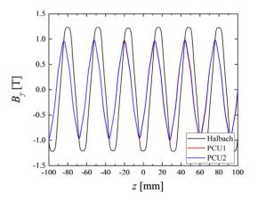
Figure 4: Measured magnetic field in the Halbach (black), PCU1 (red) and PCU2 (blue) at the gap of 4 mm. Results only near the undulator center are shown.
