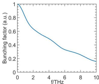
Figure 5: The beam bunching factor after chicane.
