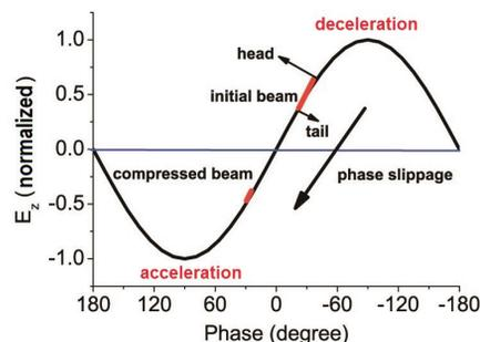
Figure 1: Principle of brake-applied velocity bunching.
