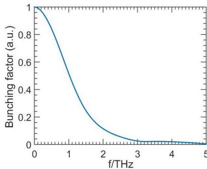
Figure 4: The beam bunching factor after BAVB.
