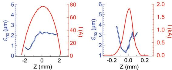
Figure 2: Slice emittance (blue) and current (red) profiles for the uncompressed (left) and compressed (right) beams.
