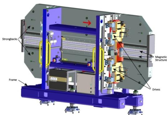
Figure 1: LCLS-II SXR Mechanical System Layout.
