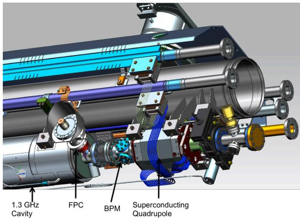
Figure 3: The end-view of the 1.3 GHz cryomodule.
