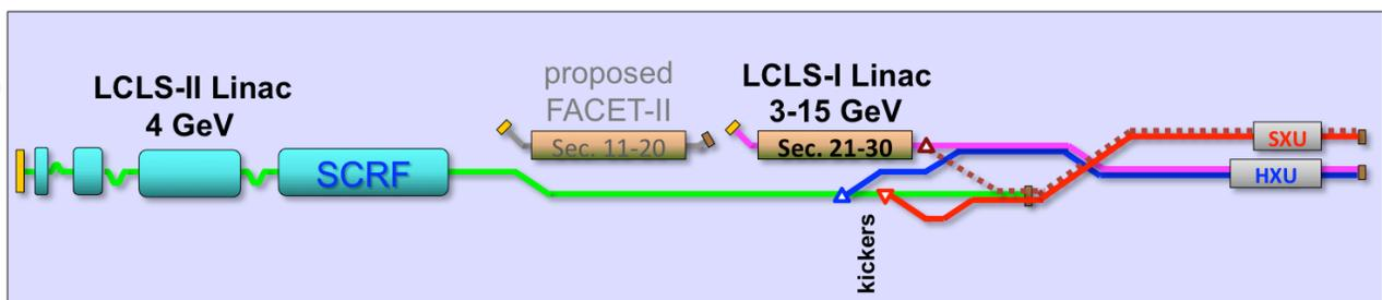
Figure 1: the LCLS-II Linac layout in the tunnel along with the existing LCLS accelerator.
