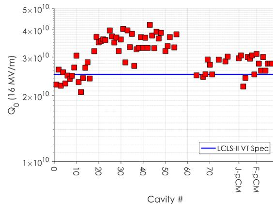
Figure 4: The Q value for the 16 cavities in the prototype cryomodules along with the Q for the cavities from vendor B for both the 800/140 and 900/200 recipe. The increase in Q from the change in temperature is clear after cavity 16.
