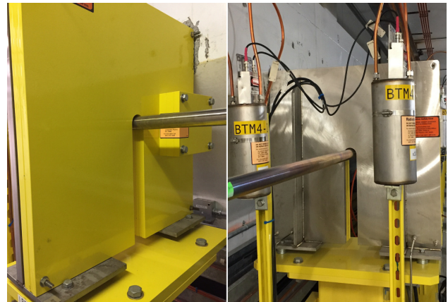
Figure 1: Front (left) and rear view (right) of an installed BTM mask at LCLS-I, instrumented also with ion chambers.
