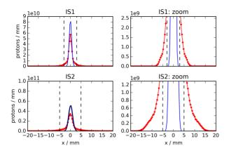
Figure 2: From LCODE [4,5] similations expected transverse profile of the self-modulated proton bunch for the AWAKE baseline parameters [3] (red) and no plasma (blue). Dashed lines indicate the size of the holes that were cut into the imaging screens (see the following section).
