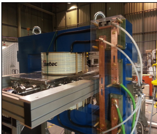
Figure 2: Vacuum chamber insert in the dipole magnet.
