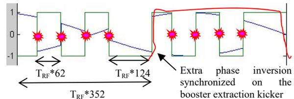
Figure 4: Example of a cleaning signal (blue) with no DC component over 2 revolutions, for  $v_H=0.25$  and four bunches (red: extraction kicker signal, pink: bunches, green: phase inversion modulation).
