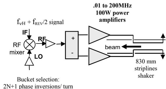
Figure 5: layout of the SY booster bunch cleaning system
