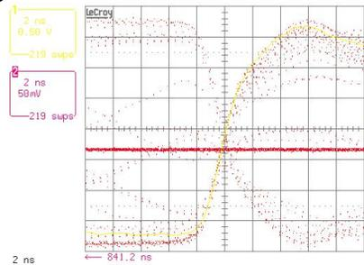
Figure 2: Kicker stripline signal rise and fall time during the phase inversions (2ns/div).
