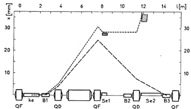
Figure 1: layout of the SY booster extraction scheme
