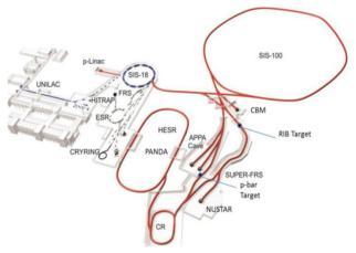
Figure 1: Layout of the existing (blue) GSI and the extended FAIR facility (red).
