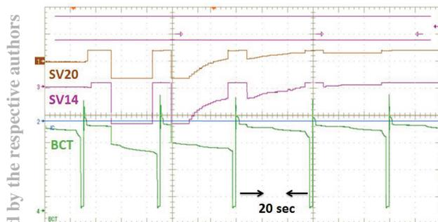
Figure 3: Exemplary oscilloscope screenshot during orbit correction. The green (lower) graph shows the beam current as function of time, indicating several machine cycles. In purple and brown the current through two vertical corrector magnets, namely SV20 and SV14 is displayed. Whereas the first cycle shows a regular ramp, during cycle number two the correction starts indicated by a step wise adjustment of the corrector current.
