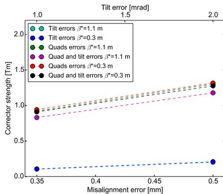
Figure 5: 90-percentile of the strength needed for the correctors on the non-crossing orbit to restore the original orbit. Cases for quadrupole misalignments and/or tilt errors are presented and for two optics:  $\beta^*=1.1$  m and 0.3 m.
