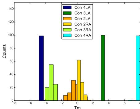
Figure 6: Distribution of the strength needed for the correctors which are used for both the correction and to provide the crossing angle. These values correspond to the case with largest misalignments and tilt errors and for the optics with  $\beta^*=0.3$  m.
