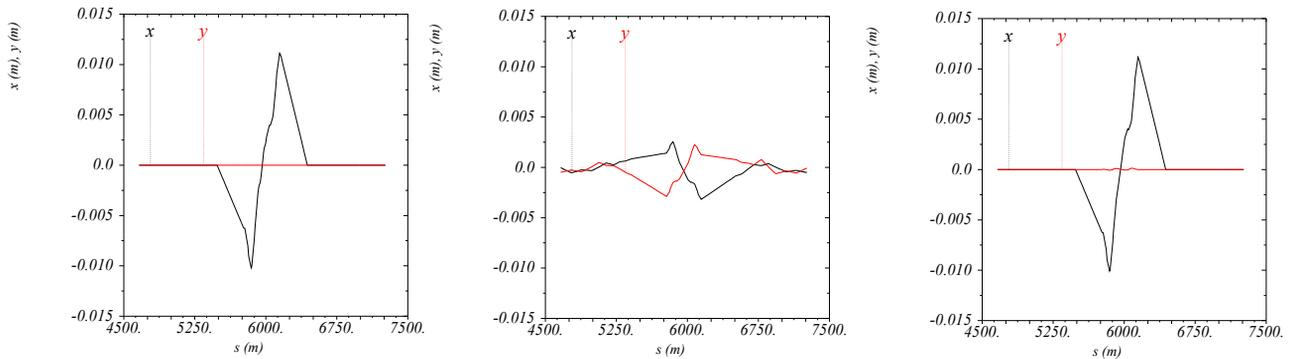
Figure 2: Representation of the correction procedure. The original orbit in IRA with horizontal crossing angle is presented at the left, when alignment errors are included the orbit gets distorted (middle) and then the correctors are used to restore the orbit as close as possible as the original one (right).
