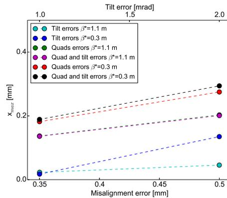
Figure 7: 90-percentile of the maximum deviation of the corrected non-crossing orbit with respect to the original orbit at the possible location of the crab cavities. Cases for quadrupole misalignments and/or tilt errors are presented and for two optics:  $\beta^*=1.1$  m and 0.3 m.
