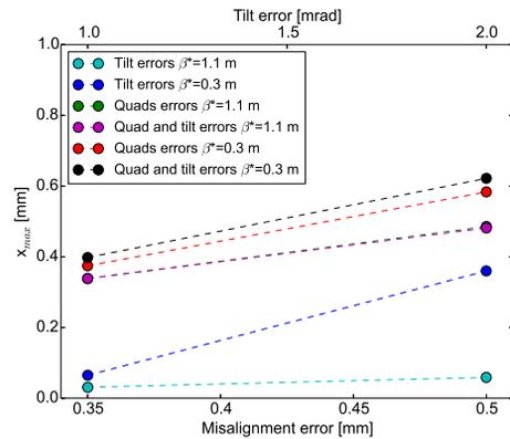
Figure 4: 90-percentile of the maximum deviation of the corrected non-crossing orbit with respect to the original orbit. Cases for quadrupole misalignments and/or tilt errors are presented and for two optics:  $\beta^*=1.1$  m and 0.3 m.
