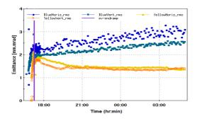
Figure 1: Beam transverse emittance evolution of the two beams for the 39 GeV/n program. The gold beam emittances in both planes (the yellow and orange) were reduced with only vertical cooling engaged.
