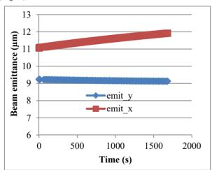
Figure 2: Transverse emittance evolution simulated by BETACOOL for the decoupled case with 9 MHz RF system; the horizontal emittance is in red and vertical emittance in blue.
