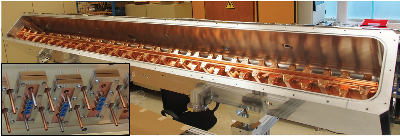
Figure 5: The MYRRHA-RFQ and water connections for stems and electrodes (small picture).
