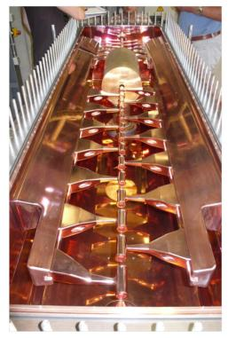
Figure 3: IH-cavity of the BNL EBIS Linac is very similar to the first IH-cavity of the heavy ion front-end [4].
