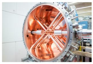
Figure 5: CH-cavity for the FRANZ Linac that is similar to the first CH-cavity of the light ion front end.
