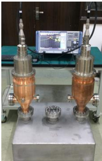
Figure 8: RF test for the two couplers of the XiPAF RFQ.
