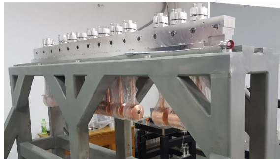
Figure 11: Drift tubes mounted on one base plate for CPHS.
