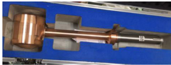
Figure 10: Drift tube successfully manufactured for CPHS of Tsinghua University.
