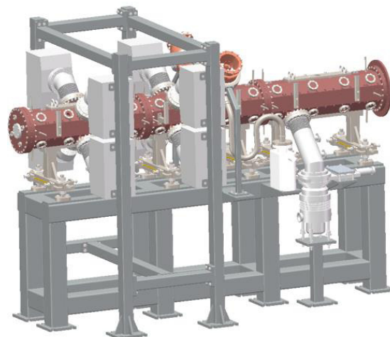
Figure 7: 3D layout of the RFQ accelerator.
