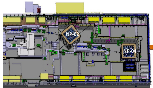
Figure 1: Layout of the extension of the EHN1 building. The two new detector prototypes (ProtoDUNE-NP02 and protoDUNE-NP-04), along with the extensions of the H2 and H4 beam lines is depicted.
