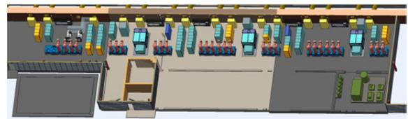
Figure 3: Klystron gallery layout for 28 new RF stations.
