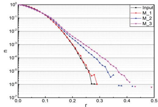
Figure 4: Phase space density plot at the end of the final FODO lattice.
