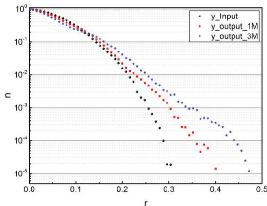
Figure 6: Phase space density plot at the end of whole beam line with measured input distribution.
