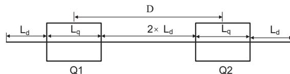
Figure 2: Lattice configuration of one FODO period.
