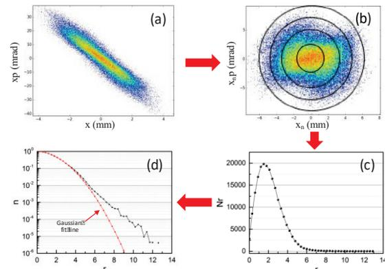
Figure 1: Transformation of a 2D phase space distribution into phase space density plot.
