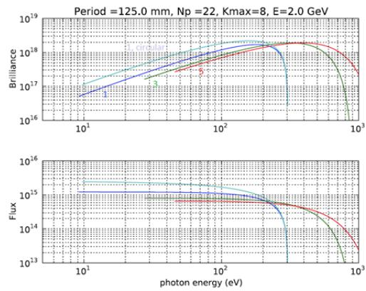
Figure 6: Characteristics, brilliance and flux of the low energy undulator for MOST.
