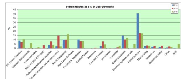
Figure 2: System failures as percentage of user downtime for 2014, 2015 and 2016.
