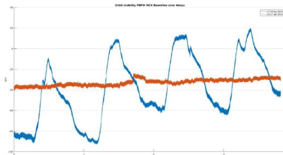
Figure 3: Photon beam stability at the MCX beam line for a period of 4 days with the air-conditioning control system on (red line) and off (blue line)
