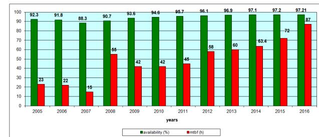
Figure 1: Combined graph of Electra availability (in %, green bars) and MTBF (in hours, red bars).
