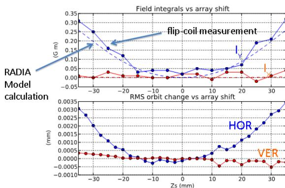
Figure 5: Calculated and measured perturbation on the electron beam orbit. The field is zero for  $Z_s$  zero.
