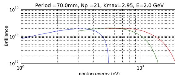
Figure 4: Brilliance in photons/sec/mm<sup>2</sup>/mrad<sup>2</sup>/0.1bw and some parameters of APU undulator
