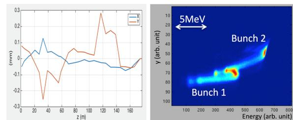
Figure 5: BPMs trajectory reading (on the left) and YAG screen image collected in the diagnostic beam dump (on the right) in two-bunch mode, when  $\Delta T=1.66$  ns.
