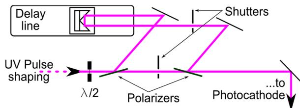
Figure 1: PIL system modified for the two-bunch operation.
