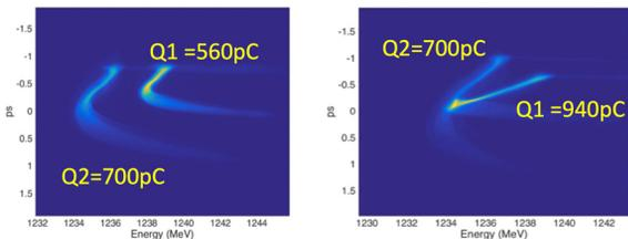
Figure 8: Longitudinal phase space of the two bunches with  $\Delta T=666$ ps, when the leader bunch has 560 pC (on the left) or 940 pC (on the right). The trailer bunch has a charge of 700 pC.
