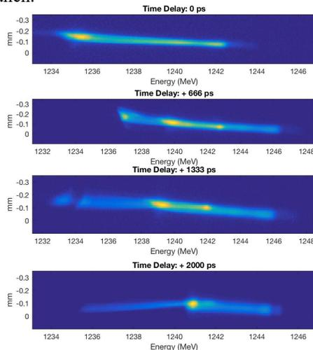
Figure 6: Energy distribution of the two bunches measured in DBD versus  $\Delta T$ . The drive bunch is on the right and the trailing one is on the left.
