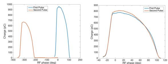
Figure 2: Schottky scan performed sending in turn only one laser pulse on the cathode. The measurement was made before (a) and after (b) the fine tuning of the temporal delay  $\Delta T$  and of the half-wave plate rotating angle.
