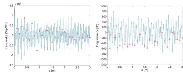
Figure 4: Simulated long-range transverse (on the left) and longitudinal (on the right) wake potential in the BTW sections. Red circles correspond to the wake potential sampled by bunches in subsequent rf buckets.
