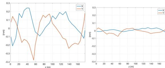
Figure 3: Second bunch (alone) trajectory along the linac before (on the left) and after (on the right) fine tuning the transverse position of the second PIL on the cathode. The reference trajectory (all reading at zero) corresponds to the first bunch trajectory obtained by sending only the first PIL pulse.
