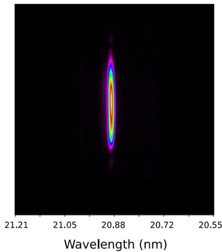
Figure 1: Spectral line of FERMI FEL-1 at harmonic 12.
